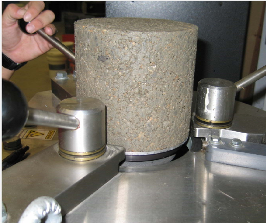
Figure 21. Extruding a Compacted RCC Specimen from the Gyrotory Compactor
